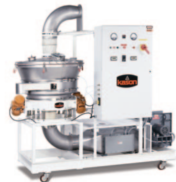
With simple connections to an existing dust collector and power source, this fluid bed dryer system is ready to reduce the moisture content of boric acid from 10 to 0.5 percent on a batch basis. It combines a 40" (1000 mm) diameter fluid bed processor, heater, blower, and controller on a caster-mounted skid.
