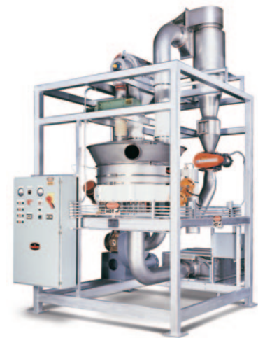
Moisture content of bulk catalyst is reduced from 9 to 1 percent at a continuous rate of 2000 lbs/h (900 kg/h) with this self-contained drying system. It is comprised of a 48" (1225 mm) fluid bed processor, heater, blower, and cyclone separator, as well as a top-mounted CENTRI-SIFTER® centrifugal screener for continuous de-agglomerating of incoming material.
