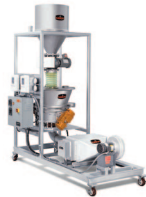
This pilot-plant-scale drying system incorporates a surge bin, rotary valve, 24" (600 mm) diameter fluid bed processor, heater, blower, and controls on a caster-mounted frame. Processors as small as 18" (450 mm) in diameter are offered for laboratory applications.
