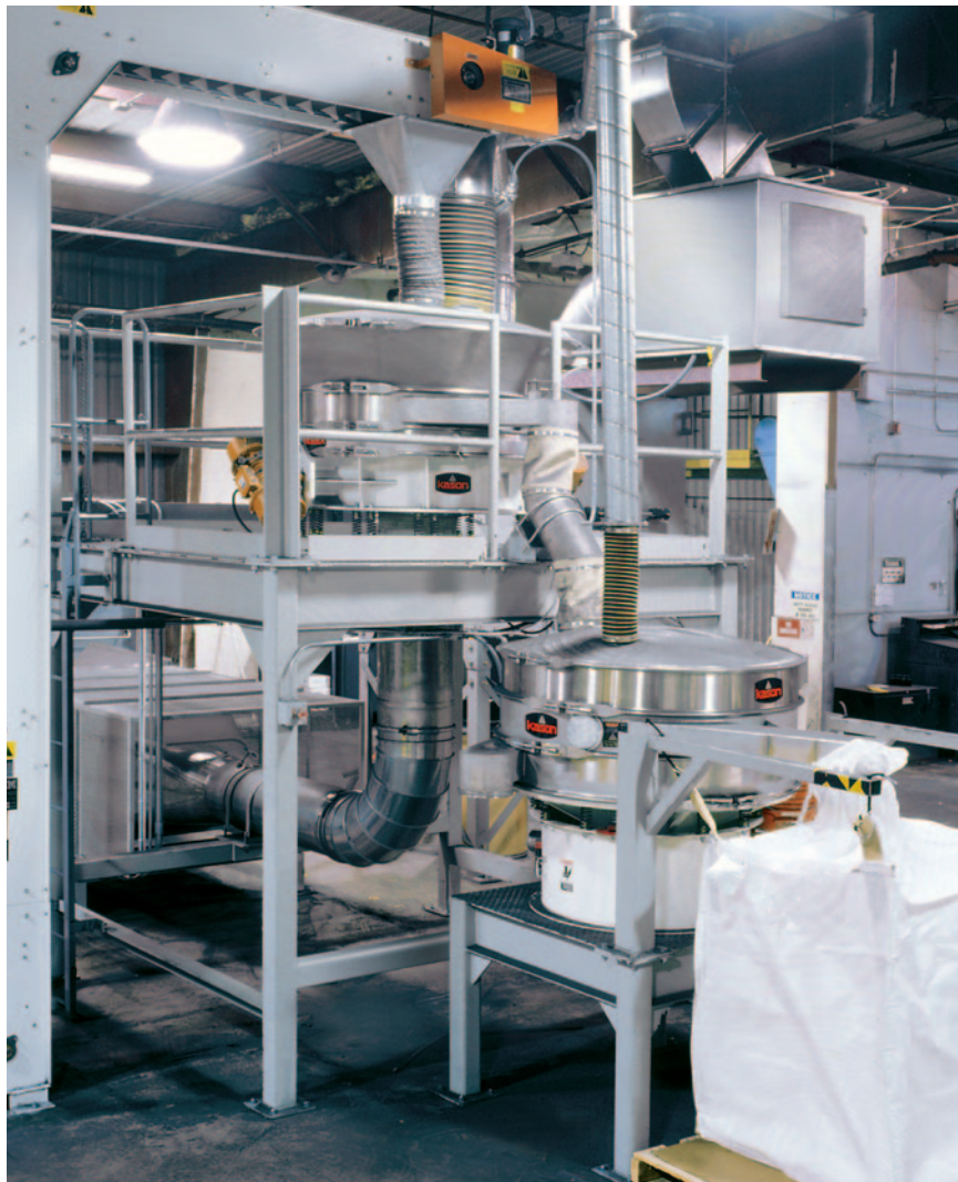
This skid-mounted, turnkey dryer-screener system configures a 48-inch (1225 mm) fluid bed dryer and two-deck circular vibratory screener in series to dry proprietary chemical powder while removing undersize and oversize particles at the rate of 2000 lbs/h (907 kg/h). The screener is equipped with a bulk bag hanger and extended discharge spout to align with the bag intake spout, and magnetic ferrule to remove tramp metal from the finished product prior to packaging.
